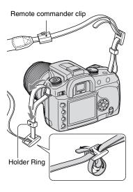
When threading the strap through the holder ring, hold the tip of the strap with your finger, as shown below, and slide the holder ring rather than the tip of the strap into position to secure the strap.
